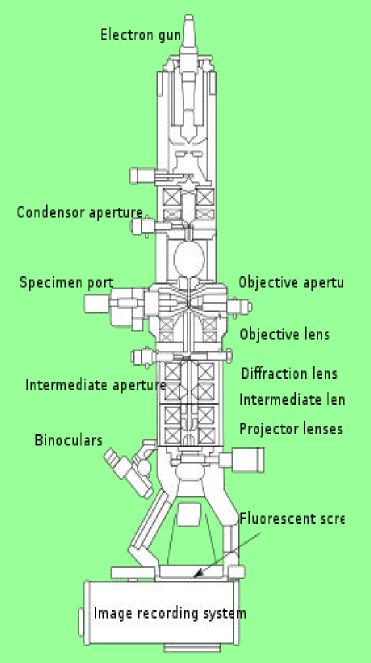
Transmission electron microscopy (TEM) is microscopy technique whereby a beam а of electrons is transmitted through an ultra thin specimen, interacting with the specimen as it passes through. An image is formed from the interaction of the electrons transmitted through the specimen; the image is magnified and focused onto an imaging device, such as a fluorescent screen, on a layer of photographic film, or to be detected by a sensor such as a CCD camera.
