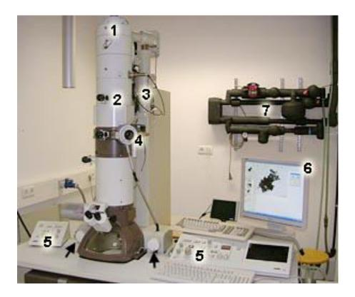
1: Electron cannon i**Transmission Electron Microscope (TEM)** n the upper part of the column. 2 Electro-magnetic lenses to direct and focus the electron beam inside the column. 3: Vacuum pumps system. 4: Opening to insert a grid with samples into the high-vacuum chamber for observation. 5: Operation panels (left for alignment; right for magnification and focussing; arrows for positioning the object inside the chamber). 6: Screen for menu and
